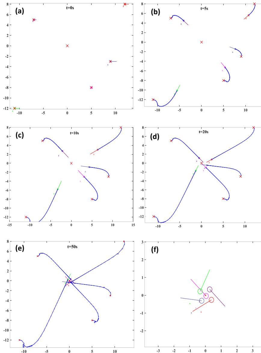
**Figure 2.** Trajectories for five WMR robots with PD controller in swarm robotics system perform a navigation control based on EBA (a)  $t = 0s$ , initial position (b)  $t = 5s$ , (c)  $t = 10s$ , (d)  $t = 20s$ , (e)  $t = 50s$ , (f) final position of 50s (2X zoom)
