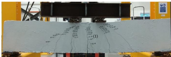
Figure 14. Failure Mode of Specimen P1
