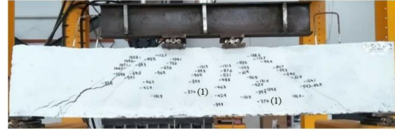
Figure 19. Failure Mode of Specimen E5/25-2
