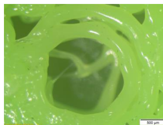
Figure 1. FDM printed micro holes (1.7 mm diameter)
