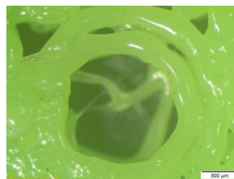
Figure 1. FDM printed micro holes (1.7 mm diameter)
