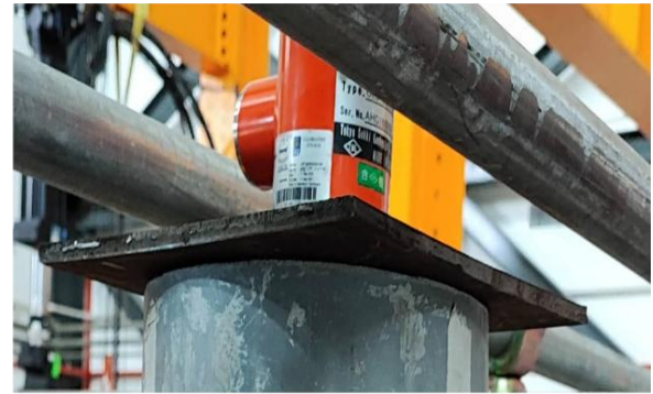
Figure 7. Failure of steel plate
