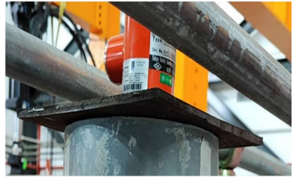
Figure 7. Failure of steel plate
