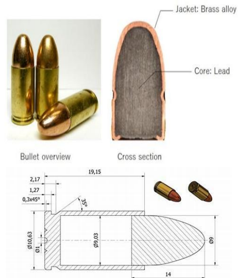
Figure 7. The 9mm bullet: A Cross-Sectional View and Dimensions
