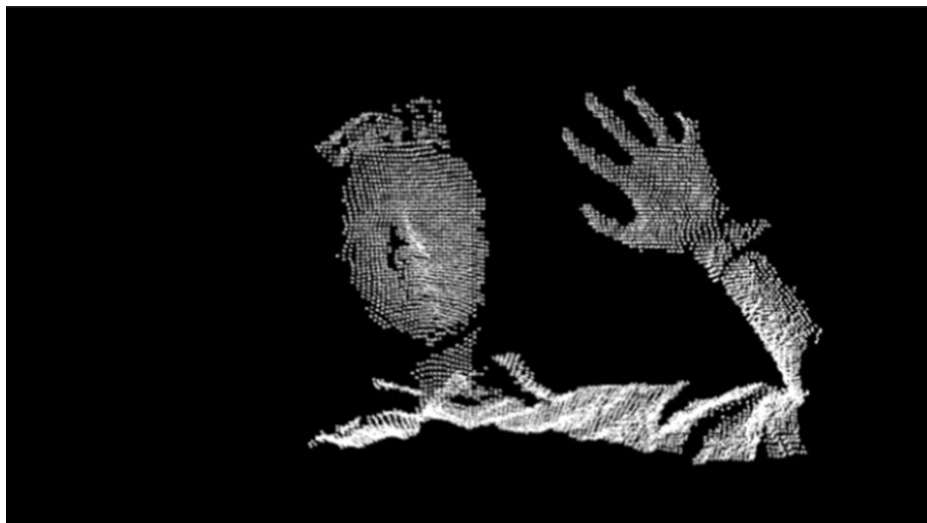
Figure 1. An example of Raw Depth Data collected by using the Kinect IR sensor and converted into visual points
